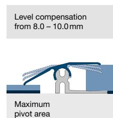
The correct laying method | **clipstech®**
