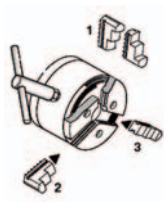
Fig. 4: Reversing or exchanging the jaws
